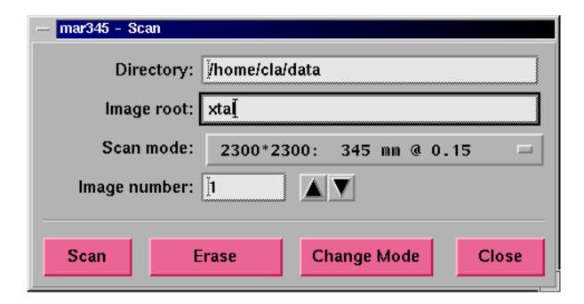
A single scan can be done by pressing the "**Scan**" button in the main window. The *mar345–Scan* window pops up. The directory, image root, image number and scan mode can be selected. The output format always is "*mar345*". Press "**Scan**" to start the scan A scan is always followed by an erase. Instead of a scan one can do an erase cycle. "Change Mode" only drives the scanning head to the desired position.
